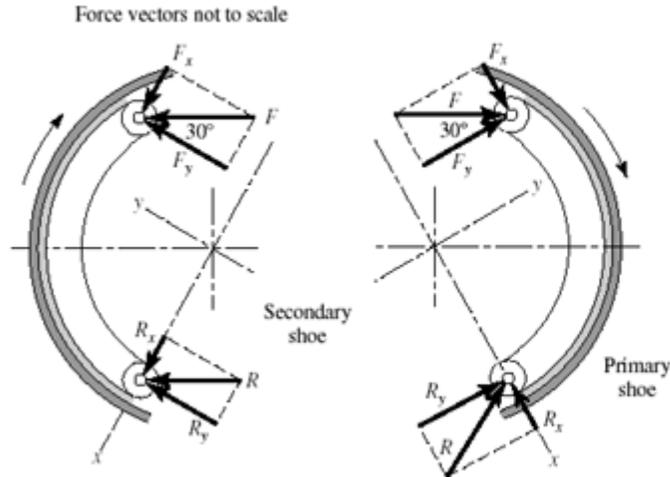
$$RH \text{ shoe: } F_x = 2200 \sin 30^\circ = 1100 \text{ N}, \quad F_y = 2200 \cos 30^\circ = 1905 \text{ N}$$
