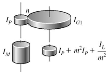
Reflect the center shaft to the motor shaft
