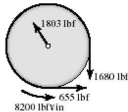
The radial load on the bearing pair is 1803 lbf. If the bearing is straddle mounted with the drum at center span, the bearing radial load is  $1803/2 = 901$  lbf.
