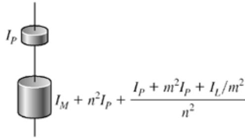
$$I_e = I_M + I_P + n^2 I_P + \frac{I_P}{n^2} + \frac{m^2}{n^2} I_P + \frac{I_L}{m^2 n^2} \quad \text{Ans.}$$
