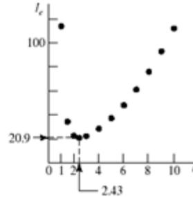
Optimizing the partitioning of a double reduction lowered the gear-train inertia to  $20.9/112 = 0.187$ , or to 19% of that of a single reduction. This includes the two additional gears.
