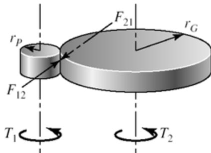
$$(T_2)_1 = -F_{21}r_p = -\frac{T_2}{r_G}r_p = \frac{T_2}{-n} \quad \text{Ans.}$$
